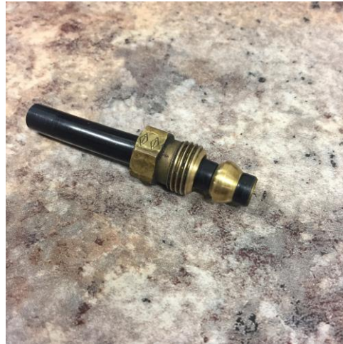
Factory Fitting after Tightening
