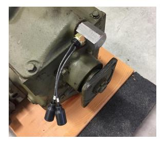
first time on the bench don't force it if resistance is felt. If the shifter doesn't want to drop smoothly into the REVERSE position remove the switch and check for any shiny spots or signs of impact with the rod. If this happens a simple thin washer will elevate the switch enough to allow a proper shift into REVERSE without resistance.
